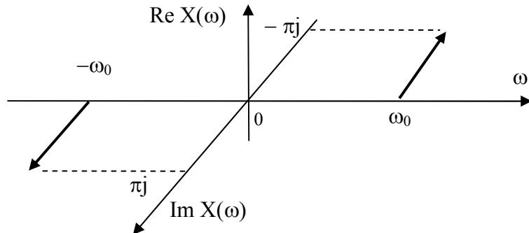
$$\begin{aligned} x(t) &= \cos(\omega_0 t + \phi_0) = \frac{e^{j(\omega_0 t + \phi_0)} + e^{-j(\omega_0 t + \phi_0)}}{2} = \frac{e^{j\phi_0}}{2} e^{j\omega_0 t} + \frac{e^{-j\phi_0}}{2} e^{-j\omega_0 t} \Leftrightarrow \\ &\Leftrightarrow X(j\omega) = \pi e^{j\phi_0} \delta(\omega - \omega_0) + \pi e^{-j\phi_0} \delta(\omega + \omega_0) \end{aligned}$$
