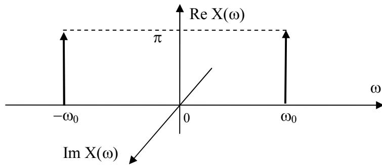
$$x(t) = \sin(\omega_0 t) = \frac{e^{j\omega_0 t} - e^{-j\omega_0 t}}{2j} \Leftrightarrow X(j\omega) = -\pi j (\delta(\omega - \omega_0) - \delta(\omega + \omega_0))$$
