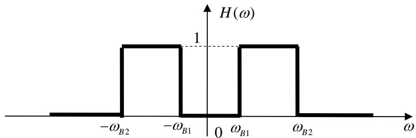
unde  $\omega_{B1} < \omega_1 < \omega_2 < \omega_{B2}$ .
