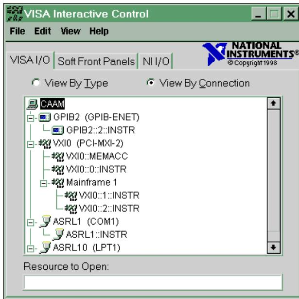
The **Soft Front Panels** tab of the main VISAIC panel gives you the option to launch the soft front panels of any *VXIplug&play* instrument drivers that have been installed on the system.
