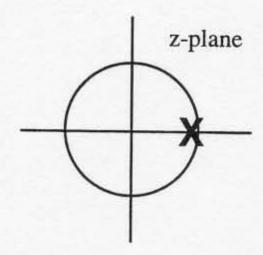
Notice that as the pole approaches the unit circle (in this example, as lal  $\rightarrow$  1), the MSE  $\rightarrow \infty$ . Thus, longer register lengths will be needed if the pole is closer to the unit circle. This observation is not unique to this example. Recursive filters having sharp transitions in their frequency response tend to have poles located very near the unit circle. Such filters require long register lengths.
