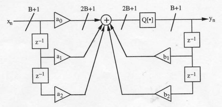
where the register lengths are indicated at various points in the filter structure. Note that the multiplier outputs have length 2B+1 and these must be quantized back to B+1 bits before they enter a feedback loop. Otherwise, the required register length will grow without bound.
