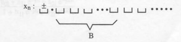
where each bit is a zero or a one. The quantizer Q rounds or truncates this representation to B bits plus sign:
