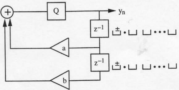
The output must be periodic in this situation because the feedback delay registers can contain only a finite number of possible pairs of values, so that at some point they must repeat. Once the contents of the delay registers repeats, the output will become periodic because the contents of the delay registers is a state of the system, which determines all future outputs.
