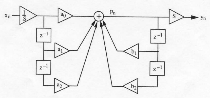
In practice, the scaling operation does not necessitate additional multiplications. S may be a power of 2, or alternatively,  $\frac{1}{S}$  can be incorporated into the  $a_i$  and you may not care whether the output is renormalized by S.
