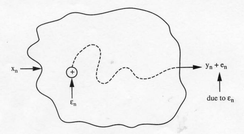
Let F(z) be the transfer function from the <u>error source</u> (quantizer) to  $y_n$ . Then for fixed-point rounding
