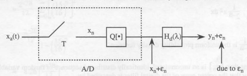
The quantizer Q is a nonlinearity. We will model it by the additive error source  $\varepsilon_n = Q[x_n] - x_n$
